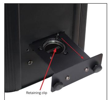
Users may change the gobos supplied for a custom design of their own. Custom gobos can be made of metal, glass or user printed onto standard transparency film. The image size for custom gobos should be no greater than 23mmØ and the overall size of the gobo should be 28.5mmØ.
