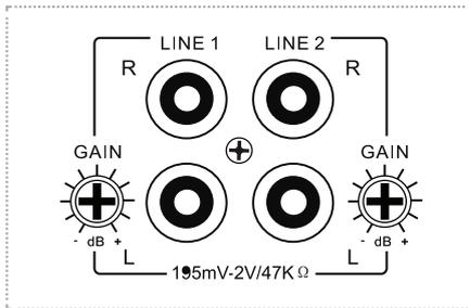
The line inputs will have an impedance of 47kΩ.
