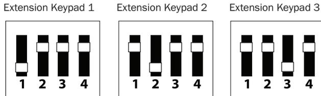
There are 4 address codes on both the remote paging console and the extension keypad which are used to identify these.
