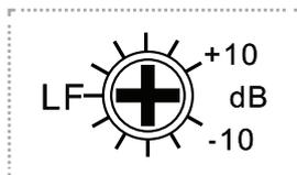
Every zone has an LF bass level control which enables the LF bass level of each zone to be set independently of other zones.
