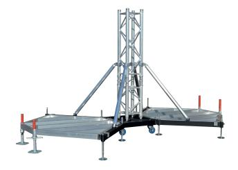
The HT tower is an upgrade on the MPT Tower, based on H3OV truss sections and employs a new type of sleeve block that fits the 40 square series truss on all four sides by means of bolted CCS6 couplers (either male or female).
