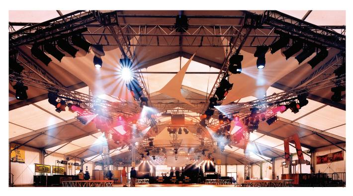
S52 Series truss is constructed of main chords (50 x 4 mm) and diagonal members (25 x 3 mm) (S52F) or 30 x 3mm (S52V and SV), and uses the CCS7 coupling system. Prolyte supplies a variety of S52 Series truss elements that provide maximum flexibility, including standard or custom-made lengths, circles and arches and several types of corners. Prolyte can create custom-made pieces on request. For obvious reasons, the S52F is not available in curved sections.
