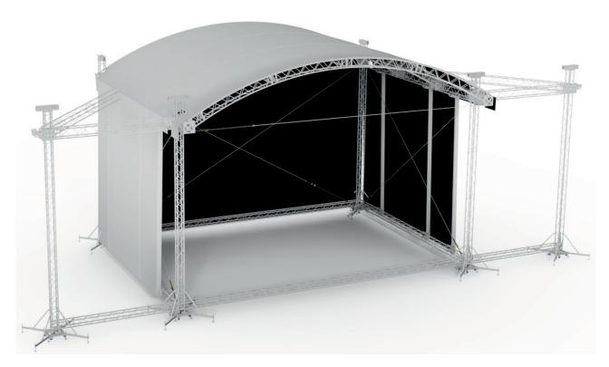
The Arc-HT roof is based on the new HT tower, the grid is build out of H40V truss and the new HD-Boxcorner which optimizes the strength of the system. The arches are made out of H40V, with compression members in-between. The HT tower simplifies the dead hanging of the system, with its dead hang pin instead of a steel chain.
