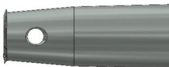
Figure 200: Mushroom head on the pin
