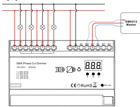
This phase dimmer adopts trailing edge dimming (reverse phase control), the dimming range is 1%~100%, please make sure the connected loads support reverse phase control. Please refer to the user manual of the load or consult the supplier of the load.
