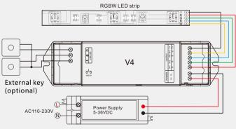
LED power supply voltage and power select: 5V Jamp, Input 5V power supply, can load 0–100W, 12V Jamp, Input 12V power supply, can load 0~240W, 24V Jamp, Input 24V power supply, can load 0~480W, 36V Jamp, Input 36V power supply, can load 0~720W, The power supply power must Jarger than load power 20%.
