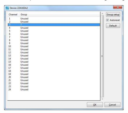
7. Click OK for save. Now you can use the channel in non-GROUP mode via front panel or when CMGxx remote is connected unit will work in group mode /more channels controlled by group control switch/
