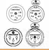
Pin 1 Pin 2 Pin 3 Ground / Common Data -Data +
