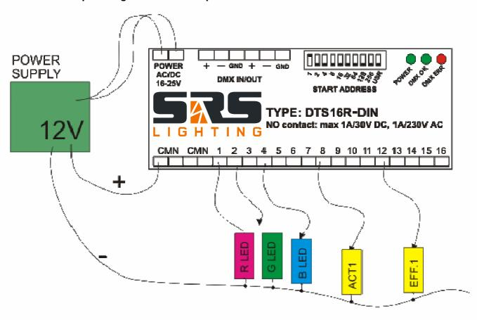
There is a 12V power supply with the output used for the load connection of LED strips and DTS16-R DIN, in the picture.
