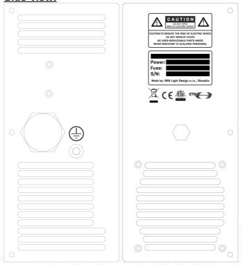
M10 mounting point for truss mount
