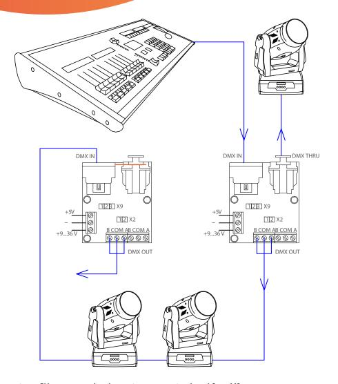
When using a 5V power supply, place a jumper on pins 1 and 2 on X9. When using a 9-36V power supply, place a jumper on pins 2 and 3 on X9.
