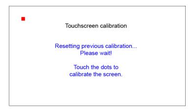
Now press the red dots to calibrate the touch screen. There will be four dots total, one in each corner of the screen. Calibration has been completed when you see the message shown above.
