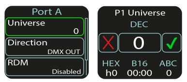
Press **SELECT**> button to access the Universe submenu. Press **SELECT**> or **SELECT**> to set the universe. Press **SELECT**> or **SELECT**> to accept.
