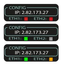
At the bottom of the home screen are two indicators. **ETH1** and **ETH2** indicate the status of the two Ethernet ports located at the back of the unit.
