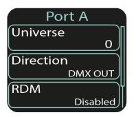
Press **SELECT>** or **SELECT>** to enter the Port submenu or **SELECT>** to return to the home screen. Select any of eight ports to set the desired values.
