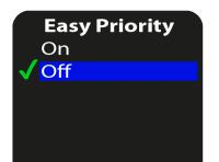
Press **<DOWN>** or **<UP>** buttons to turn the Easy Priority ON or OFF. Press **<SELECT>** or **<RIGHT>** to set or **<LEFT>** to decline. Press **<LEFT>** to return to the home screen.
