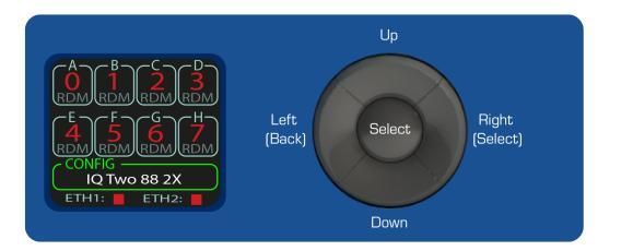
Access Main menu functions using the navigation pad next to the LCD display.
