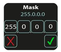
Press **<UP>** or **<DOWN>** to change value for each highlighted window. Press **<LEFT>** or **<RIGHT>** to navigate selection window. Press **<DOWN>** and then **<LEFT>** or **<RIGHT>** to decline or confirm, **<SELECT> >** to accept changes.
