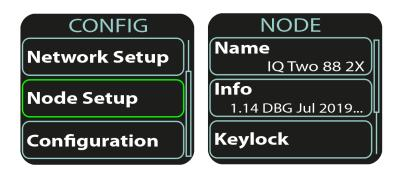
Press **SELECT** or **SELECT** to enter the Node Setup submenu or **SELECT** to return to the home screen.
