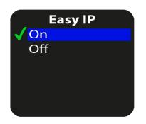
Press **<DOWN>** or **<UP>** to turn the Easy IP ON or OFF. Press **<SELECT>** or **<RIGHT>** to set or **<LEFT>** to decline. Press **<LEFT>** to return to the home screen.
