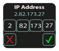
Press **<UP>** or **<DOWN>** to change value for each highlighted window. Press **<LEFT>** or **<RIGHT>** to navigate selection window. Press **<DOWN>** and then **<LEFT>** or **<RIGHT>** to decline or confirm, **<SELECT>** to accept changes for the IP address.
