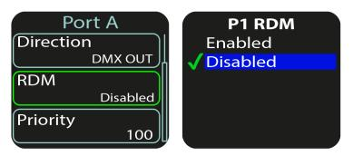
Press **<SELECT>** to access the RDM submenu. Press **<UP>** or **<DOWN>** to enable or disable RDM function. Press **<SELECT>** or **<RIGHT>** to accept, **<LEFT>** to decline changes.
