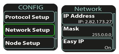
Press **SELECT** or **SELECT** to enter the Network Setup submenu or **SELECT** to return to the home screen.
