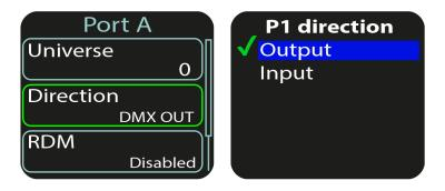
Press **<SELECT>** to access the DMX Direction submenu.
