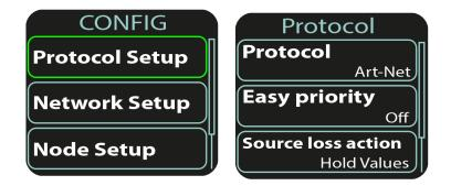
While in the home screen, press any of directional buttons to activate selection window. Navigate selection window to CONFIG and press <SELECT> to access CONFIG submenu. Press <SELECT> or <RIGHT> to enter the Protocol Setup submenu or <LEFT> to return to the home screen.
