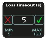
Press **<UP>** or **<DOWN>** to set Source loss timeout (5-120s) Press **<LEFT>** or **<RIGHT>** to decline or confirm, **<SELECT>** to accept.
