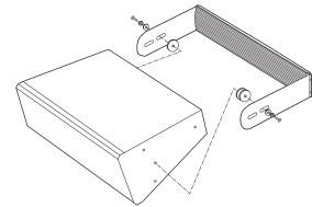
**7.** Rotate the speaker to the desired direction then fully secure the side bolts.
