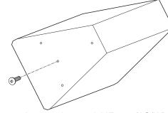
If you are using speaker model IF2112/AS(W), install the socket cover bracket to the speaker using the M10 button head screws.
