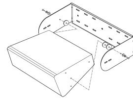
**6.** Rotate the speaker to the desired direction then fully secure the side bolts.
