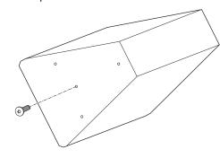
If you are using speaker model IF2115/AS(W) install the socket cover bracket to the speaker using the M10 button head screws.
