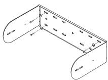
**5.** Rosition the speaker in between the bracket arms with the sound isolation gaskets. (Use one each of the 1/4" and 1/8" gaskets on one side and one 1/4" gasket on the other side.) Secure the speaker to the bracket using the included hardware through the desired slots into the speaker enclosure's threaded mounting holes.
