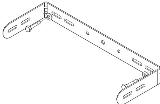
5. Position the speaker in between the bracket arms with the sound isolation gaskets. Secure the speaker to the bracket using the included hardware through the desired slots into the speaker enclosure's threaded mounting holes.
