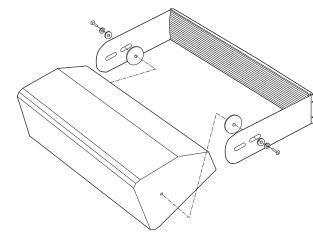
**7.**Rotate the speaker to the desired direction then fully secure the side bolts.
