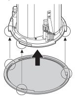
CAUTION The grille may fall down if it is attached inadequately. Attach it firmly.
