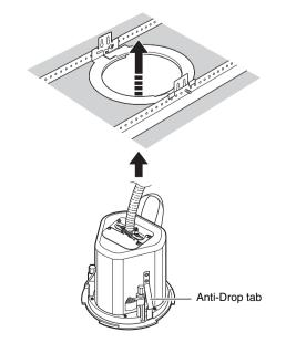
To release the speaker from the O-ring, press the Anti-Drop tabs. These are located above the  $\blacktriangle$ mark near the edge of the cabinet's face.
