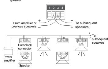
4 Plug the connected Euroblock connector into the socket in the speaker
